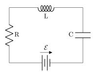
Let  $\mathcal{E}$  be the voltage of the battery, R be the resistance of the resistor, C be the capacitance of the capacitor, and L be the inductance of the inductor. Using Kirchhoff's Law, we have
